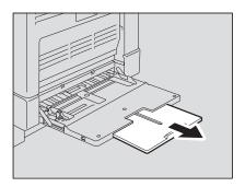
Check if the lamp of the paper size placed on bypass tray is lit. If not, press the [COPY] button several times until the lamp of the desired paper size is lit.
